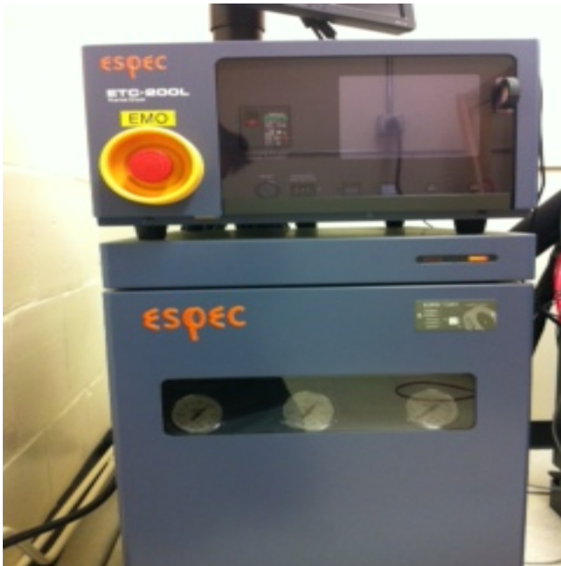
Figure 1-8 Temperature Control Unit
